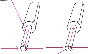
Engage the locking mechanism on the roll holder and slide it into your media. Make sure that the media holder is at the correct width of your media. Place the media back into the drawer.
