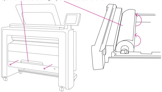
Lift roll up and out of drawer, and place on the loading station.
