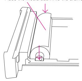
Gently roll the media so the edge feeds under the roll and into the paper guide. The printer should automatically grab the roll.
